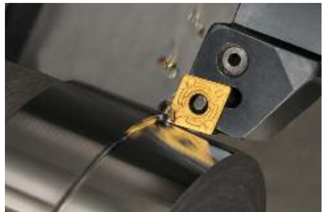
High feed turning at high speeds with NGE type chipbreaker (Coated grade: AC810P)
